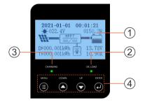
1.LCD Display2.DC Load Indicator3.Charging Indicator
