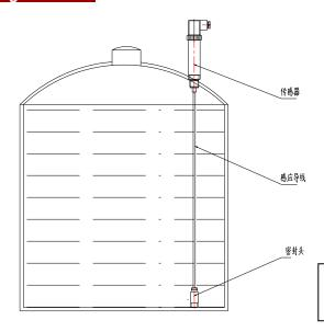
Mount with flange or screw thread on the closed container
